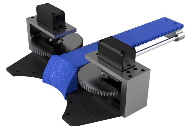
make the system faster and also changed the servomotors from high-torque to high-speed. The latter change made a big difference to how the system worked, speeding the push-pull time from 2 seconds to 0.5 seconds. Also, we bought some new bearings that were recommended to us by an engineer at Wenglor, and all that we can say is that the difference was enormous for the difference in price.
